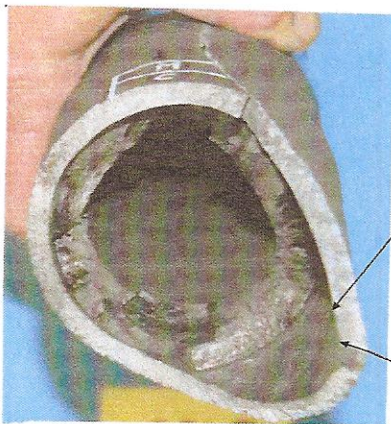
Cokified Furnace Tube
