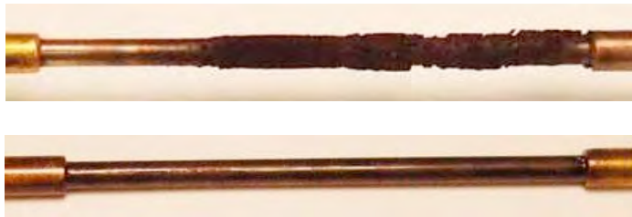
Figure 8. Uncoated (top) and C3 nanofilm coated (bottom) alloy tube exposed to residual oil on the outside, while being heated by heaters inside the tubes. Note that the C3 coated tube has much less, and more uniform, coke buildup.
